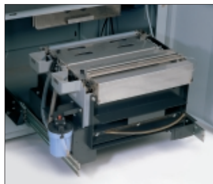
Self-replenishing plate processor has easy-access, deep tanks that constantly recirculate to extend chemistry life.
